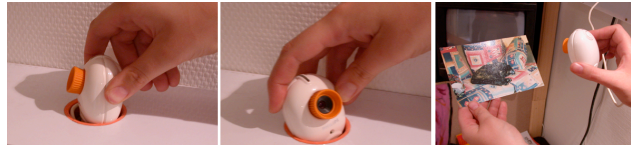
Figure 2: The video camera can be turned or used to actively take a photograph of a particular object.
