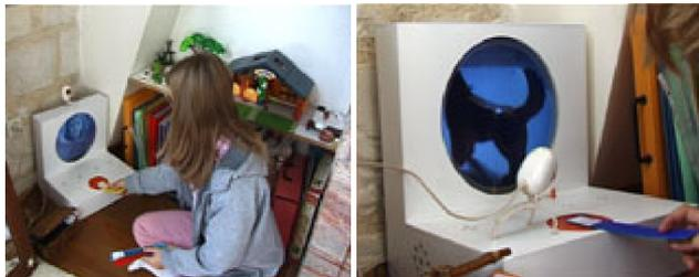
**Figure 8: StoryTable has a tangible interface to record, play and share video clips captured with the local camera.**
