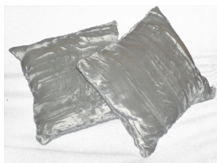
Figure 4 : Augmented cushions: both cushions measure the pressure applied to them and vibrate according to the pressure applied to the other one
