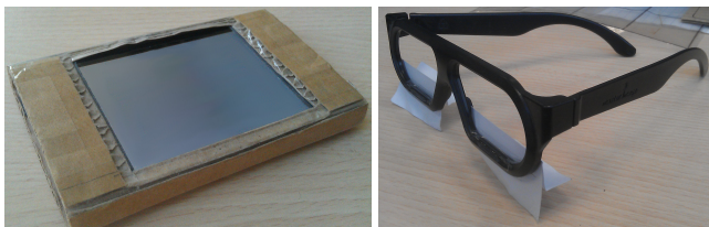
Figure 1: The cardboard overlay covering the iPod Touch (left) prevented touch detection outside the open area. The blinder glasses (right) were made from plastic ones by taping pieces of paper at their bottom.
